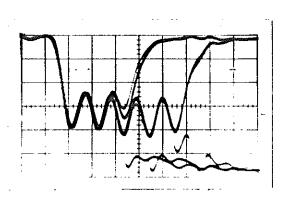
FIGURE 2. Sampling and real-time oscilloscope displays of the response of a TTL R-S flip-flop (constructed by cross-tying two SN7400 NAND gates) to both inputs being changed HIGH simultaneously (sampling displays) and to a weak pulse applied to one input (real-time displays). 5 nsec./div., lV/div. for sampling displays; 10 nsec./div., lV/div. for real-time displays.
