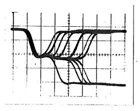
FIGURE 1. Sampling and real-time oscilloscope displays of the response of an ECL clocked R-S flip-flop (Motorola MC1016) to the clock input signal being switched off as the data input signal is changing. 5 nsec./div., 0.25V/div. for sampling displays; 10 nsec./div., 0.2V/div. for real-time displays.
